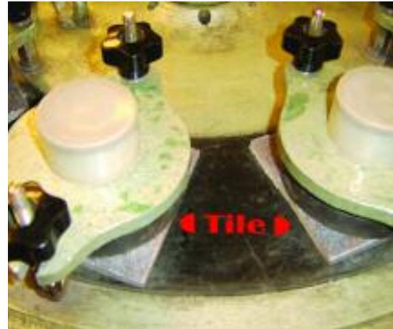
**Above:** This picture shows the mechanical device used to present swirling abrasive media to the glazed surface of the tiles.
