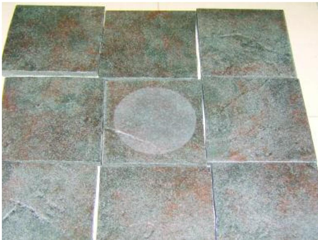
**Right: The ASTM C-1027 test procedure for glazed tile surfaces entails four-inch tile squares subjected to swirling abrasive media on the tile's surface. A calibrated light box is used to visually compare the center tile to the surrounding unabraded tiles for surface damage. Surface wear is detected visually from a designated distance and viewing angle.**
