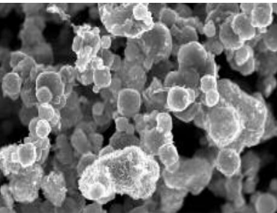
**Above: Photograph of ceramic tile raw material at 10,000 X magnification. Photograph taken by the National Brick Research Center.**
