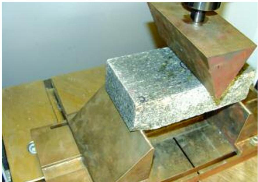
**Figure 1: ASTM C99 Modulus of Rupture establishes the bending strength of the material using a three-point beam loading fixture.**
