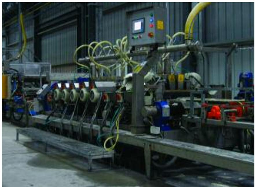
**Right: Tile rectification commonly involves equipment with precision saws and grinders.**
