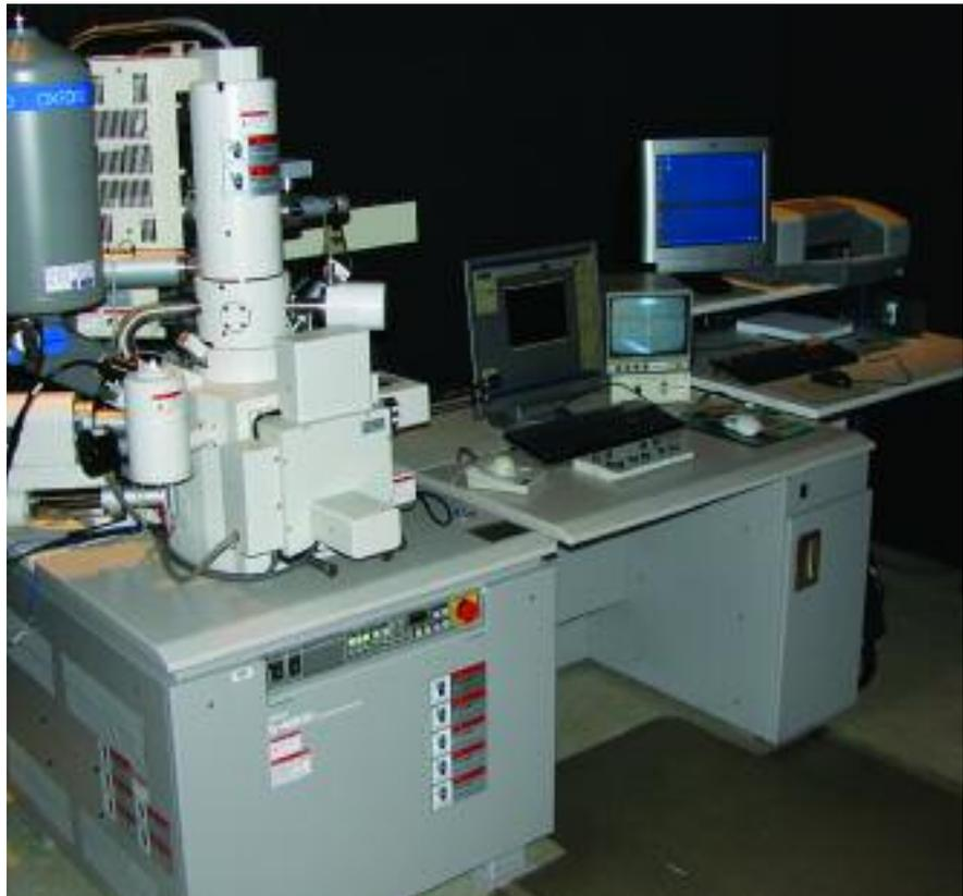
**A scanning electron microscope gives three-dimensional images over a wide range of magnification, allowing examination and measurement of surface features such as cracks, pits, and inclusions. Photo courtesy of Clemson University.**
