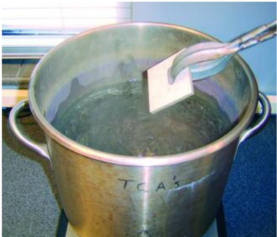
**More rigorous than the prescribed ISO test method, ASTM C373 requires a rapid five-hour boil followed by a 24-hour soak.**
