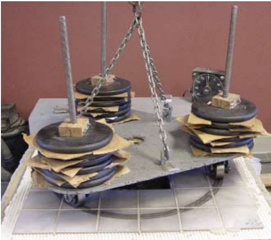
Above: The assembly pictured above is on cycle number 12. Once the cart has completed the 450 revolutions required by cycle 12, the sample will undergo a visual examination to determine whether or not cycle 13 will commence.
