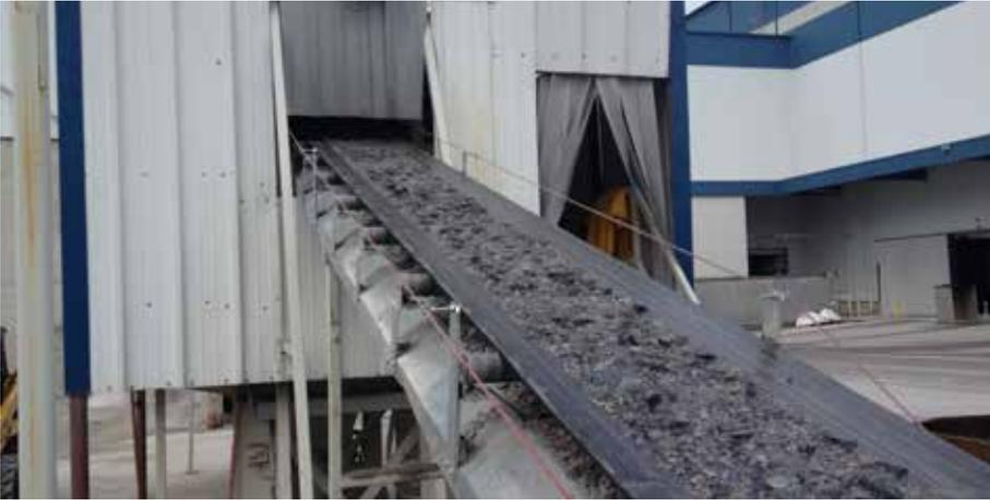
*In addition to pre- and post-consumer recycled content, high levels of responsibly-recovered waste including dust, powder, fired and unfired scrap, and water are commonly reincorporated into tile manufacturing processes which can result in true closed-loop manufacturing.*
